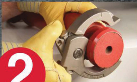
Push collar onto bolt
